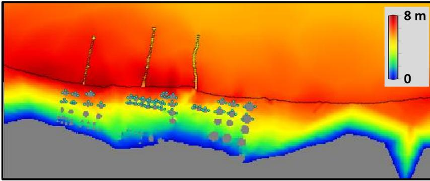
**FIGURE 7:** Example of a high-resolution tsunami inundation map showing the maximum wave height in the Milazzo Port, southern Italy, for a nearby magnitude 8 earthquake.
