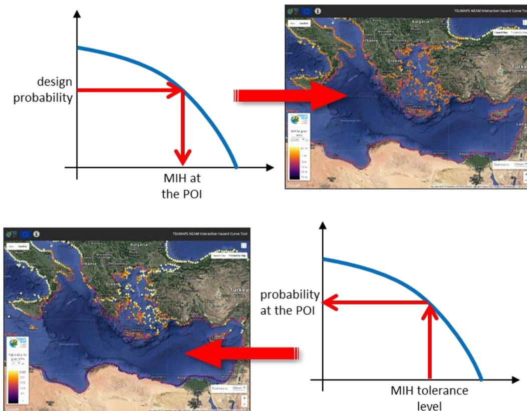
**FIGURE 6: Top, a hazard map, i.e. the values of MIH in meters at each POI, obtained by cutting the hazard curves at a given probability of exceedance in 50 years; Bottom, a probability map, i.e. the probability of exceedance in 50 years, obtained by cutting the hazard curves at a given MIH value.**
