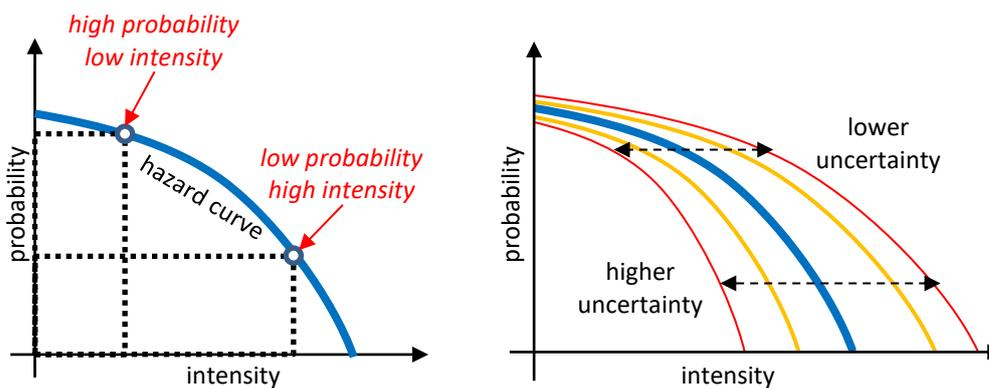
**FIGURE 5: Left, a sketch of a hazard curve; Right, a sketch of a suite of percentiles expressing the uncertainty of the hazard model.**
